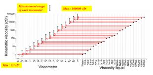
Figure 2: The range of each viscometer in step up procedure and the viscosity value of the viscosity liquid matched to each viscometer
