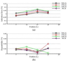
**Figure 5:** Device 1, the indication error (a) and repeatability (b) of different experimental sections of the piston cylinder at different flow rates with a verification volume of 6 L.
