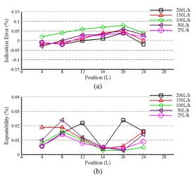
**Figure 3:** Device 1, the indication error (a) and repeatability (b) of different experimental sections of the piston cylinder at different flow rates with a verification volume of 4 L.
