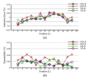
**Figure 2:** Device 2, the indication error (a) and repeatability (b) of different experimental sections of the piston cylinder at different flow rates with a verification volume of 2 L.
