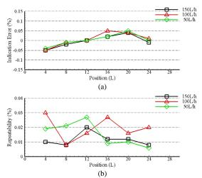
**Figure 4:** Device 2, the indication error (a) and repeatability (b) of different experimental sections of the piston cylinder at different flow rates with a verification volume of 4 L.
