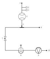
Figure 4: The roots flow-meter measurement part of the flow standard device
