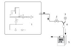
Figure 2: The load performance test deviceNote: 1-The flow standard device, 2-The pressure regulating valve,3-The electronic pressure gauge, 4-The tee, 5-The ambient air sampler
