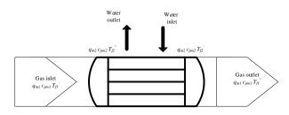
Figure 4: Schematic diagram of heat exchange treatment of the facility
