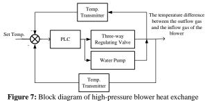
gure 7: Block diagram of high-pressure blower heat exchang subsystem
