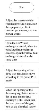
Figure 10: Workflow of Heat Exchanger Subsystem
