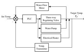
Figure 9: Block diagram of heat exchange system
