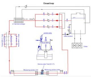
Figure 2 Closed Loop and DUT Calibration
