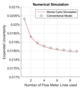
Figure 9 Results of a multivariate correlated Monte Carlo Simulation using experimentally determined covariances.
