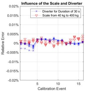
Figure 10 Performance of the diverter system and the weighing scale for the analysed 6-month period. The errors between calibrations are very low. No influence on the master calibration is expected
