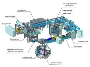
Figure 1 Schematic diagram of the FCP-25
