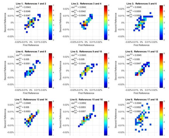
Figure 5 Calibration results for all flowmeter pairs. The colourmap represents the occurrences of the result in each box. In contrast to a Youden plot, this representation attempts to represent the frequency distribution.
