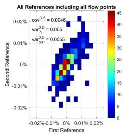
Figure 6 Calibration results given for all flowmeter pairs and all flow points
