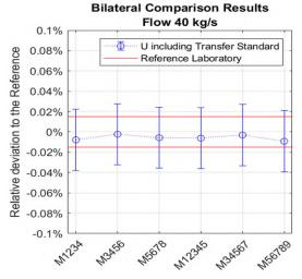
Figure 13 Bilateral comparison at 40 kg/s compared to FCP-7.1.5 described under [3]. The error bars include the Transfer Standard. Consistency is clearly given.
