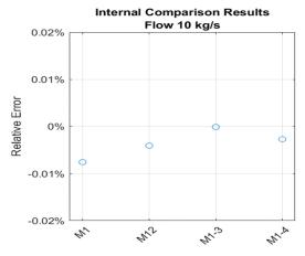
Figure 11 Internal comparison between different reference flowmeter configurations using 1, 2, 3 and 4 lines.
