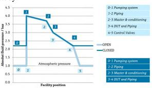
Figure 4 Fluid pressure within the calibration facility
