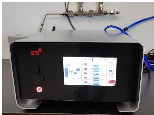
Figure 2: The completed development of the laminar flow device
