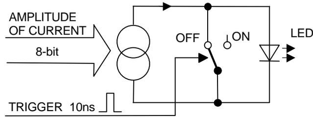
**Figure 2.** Principal functional diagram of the DOC based on digitally-controlled current source and high-speed switch.
