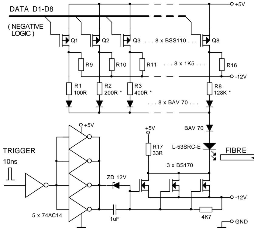
**Figure 3.** Practical implementation of the DOC for Programmable photostimulator PPS-1.
