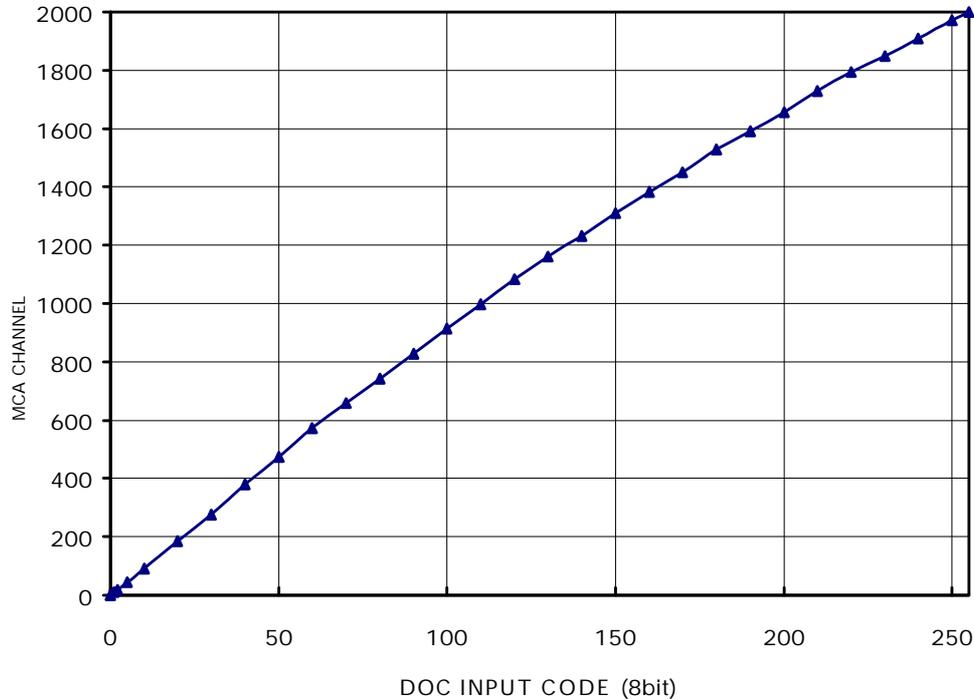
**Figure 4.** Digital-to-optical conversion characteristic with the L-53SRC-E LED-diode.
