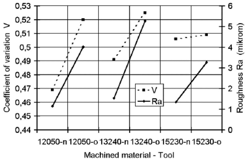
Figure 5. Roughness Ra and coefficient V dependence upon tool wear (turning)
