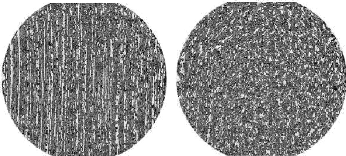
**Figure 2.** Drilled steel 15230.3 surface morphology (sharp and worn-out tool)
