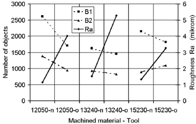
Figure 3. Influence of tool wear upon number of objects in turning (n-new tool, o-worn tool)
