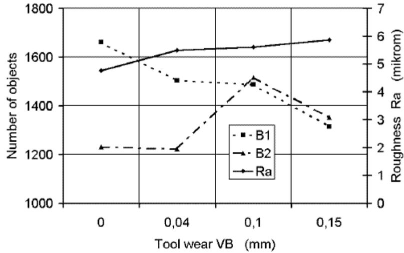
Figure 4. Influence of tool wear upon number of objects in drilling
