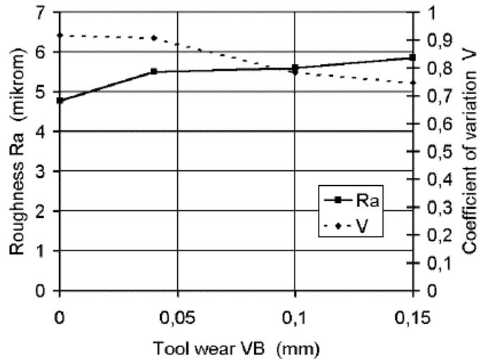
Figure 6. Roughness Ra and coefficient V dependence upon tool wear (drilling)
