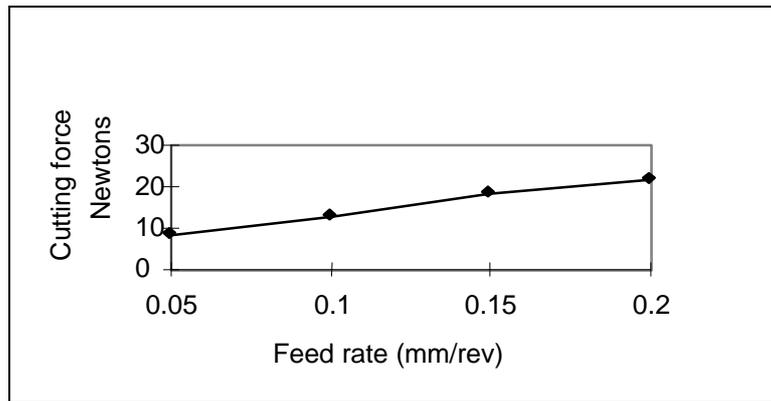
Figure 5. Effect of feed rate on cutting force.
