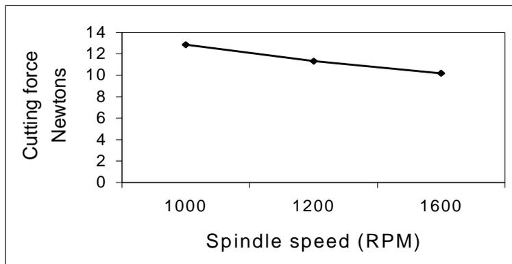
Figure 9. Effect of spindle speed on cutting force
