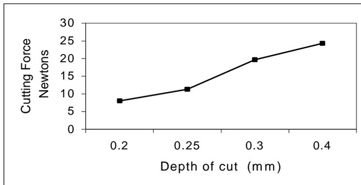
Figure 6. Effect of Depth of cut on cutting force
