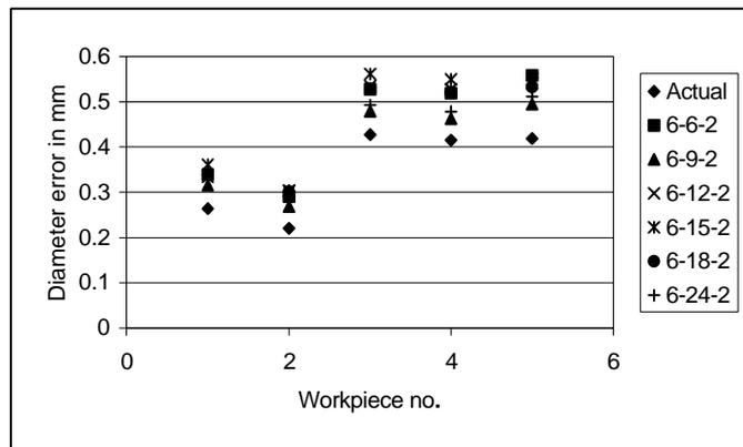
Figure 2. Effect of No. Hidden Nodes on the Error for 50k cycles
