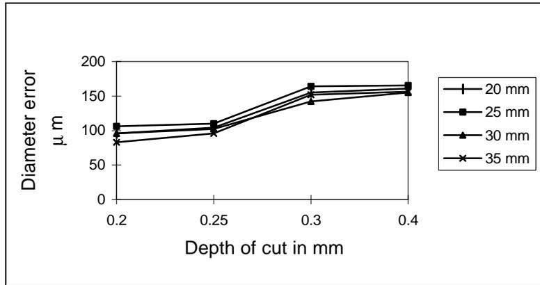
Figure 8. Effect of Depth of cut on the diameter error
