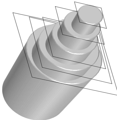
**Figure 4.** Planes along which the Form errors were measured
