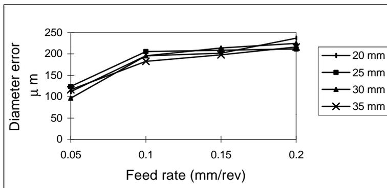
Figure 7. Effect of Feed rate on Diameter error
