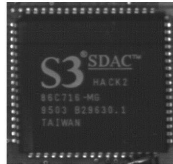
Figure 4. Detailed image of an IC, obtained with the high-resolution line-scan camera.
