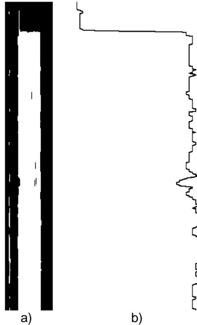
**Figure 5.** Column width measurement: a) the thermometer column after image processing. b) the column vertical profile.
