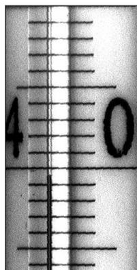
**Figure 8.** Thermometer with a thin column
