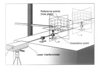
Fig. 4. The concept of transposing a matrix method for large machines
