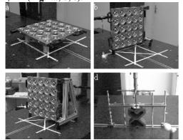
Fig. 2. Sequence of a plate positions assumed for determination of the reference grid: situation a) XY, b) YZ c) YZ in the consecutive position d) determination of FBG for the head.
