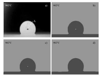
Fig. 3 Original image of specimen of silver (a) and results of its segmentation (b, c, d). (A – object removed in segmentation process)
