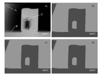
Fig. 2 Original image of specimen of glass (a) and results of its segmentation (b, c, d).
