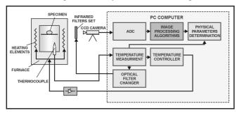
Fig. 1. Block diagram of computerised system with CCD camera for measurement of surface properties
