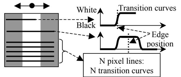
Fig. 3 One or two edge targets and single or multiple pixel line analysis
