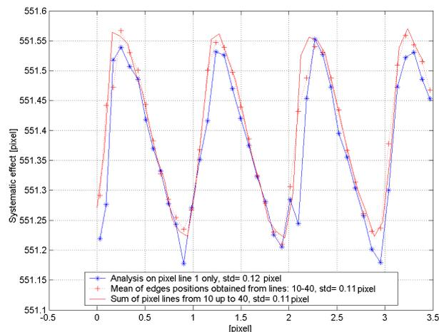
Fig. 6 Systematic effect considering one pixel line or 30 pixel lines with the standard and the new proposed approach
