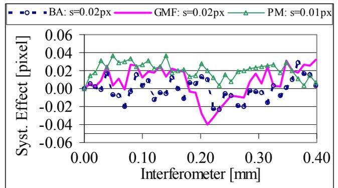
Fig. 11: Systematic effect with rhomboid target (square target 45° rotated)
