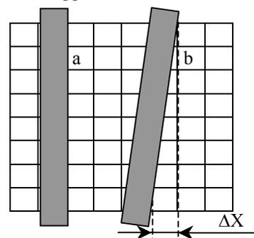
Fig. 4 Target edges parallel or angled with respect to the pixel grid
