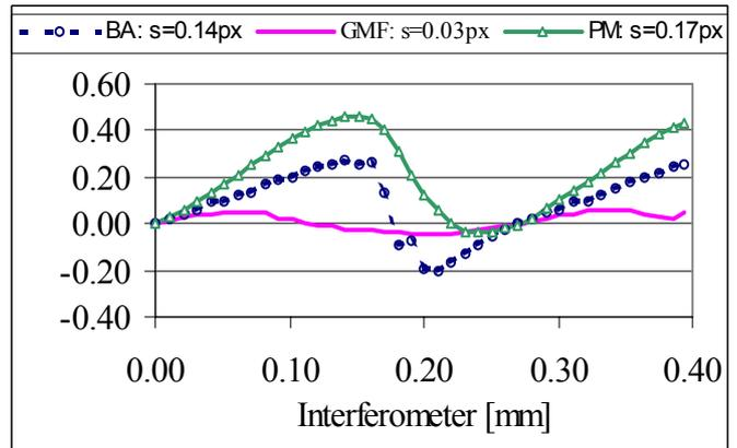
Fig. 10: Systematic effect with rectangular target with sides parallel to the pixel grid
