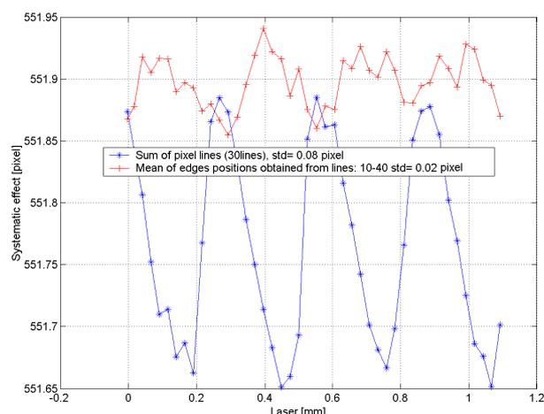
Fig. 7: Systematic effect in case of 2.1° rotated rectangular target
