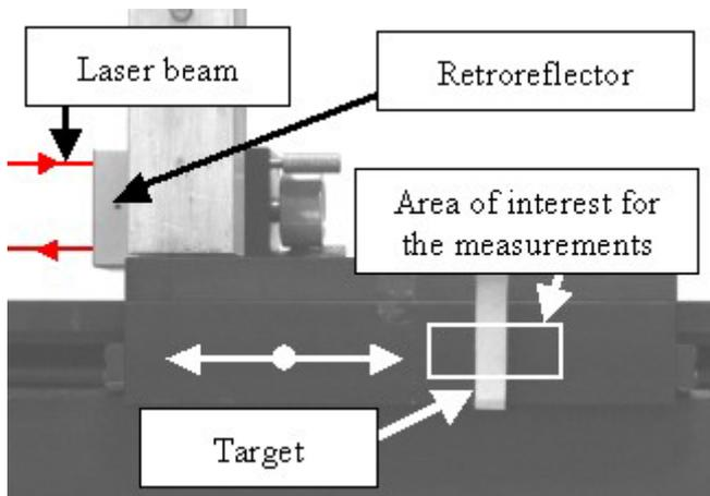
Fig. 2 Sliding support of the target and laser interferometer retroreflector (viewed from the camera under test)
