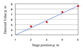
Fig.12 Experimental result of horizontal displacement measurement
