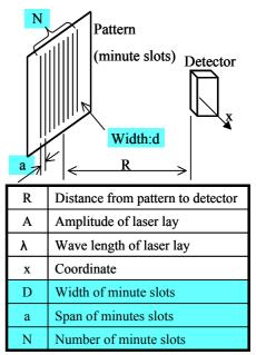
Fig.7 Parameters of Fraunhofer diffraction equation
