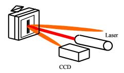
Fig.11 Experimental device for horizontal displacement measurement
