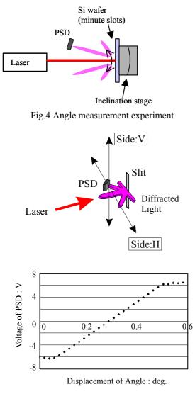
Fig.5 Angle displacement measurement precision
