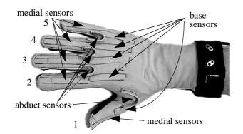
Fig. 2. Picture of the cyberglove, name of the sensors and fingers numbering
