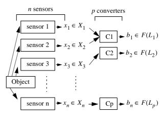
Fig. 3. Structure of a fuzzy sensor
