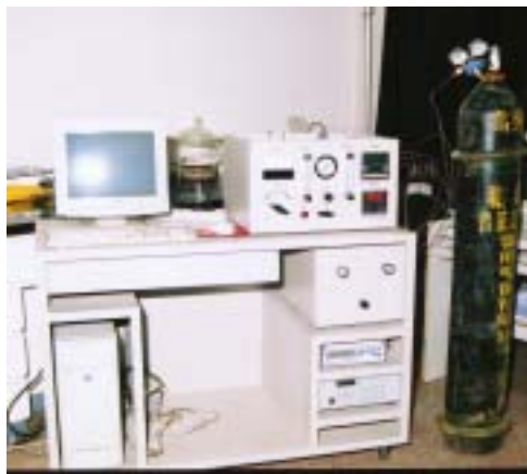
Fig. 2. The dynamic volumetric method apparatus
