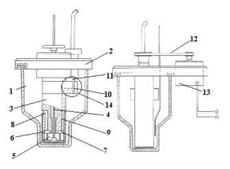
Fig. 2. Electrochemical vessel structure
