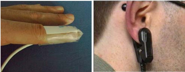
Fig. 14. IR PPG finger and ear-lobe sensors used for monitoring
