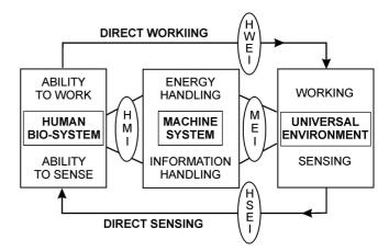
Fig.2 Interface between humans, machines and the universal environment [4]. HMI- Human Machine Interface, HWEI – Human Working Environment Interface, MEI – Machine Environment Interface; HSEI – Human Sensing Environment Interface.
