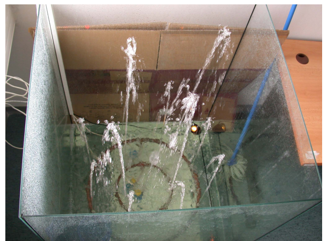
Fig. 5. Cubical aquarium with three circuits with nozzles
