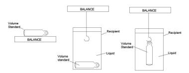
Fig. 2. Second assembling of hydrostatic weighing system
