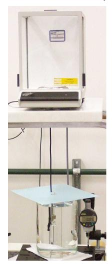
Fig. 3. Second assembling of hydrostatic weighing system
