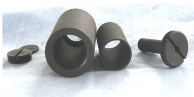
Fig. 1: Photograph of a typical high temperature fixed point crucible
