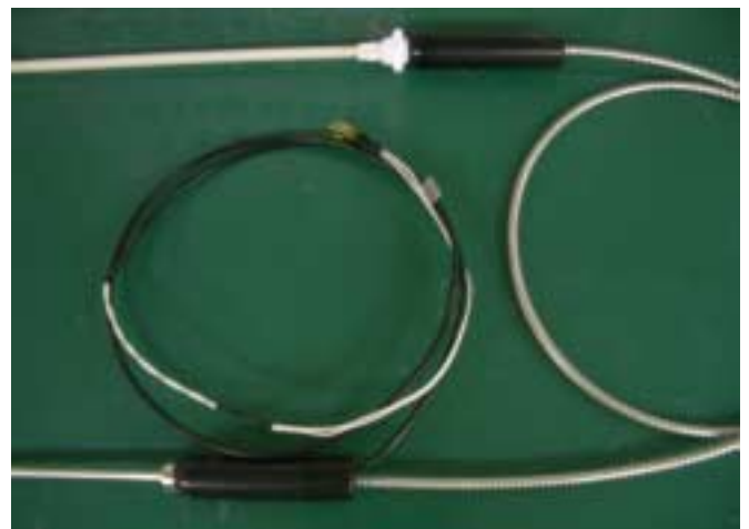
Fig.11 Picture of the thermocouple. In the handle of Ice point probe, thermocouple wire is anchored. Flexible stainless bellows connecting thermocouple and reference junction protects thermocouple wire from any stress for the thermocouple.
