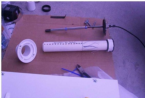
Fig. 2. Photograph of warmed probe and a “field expedient” baffle fabricated on site from PVC pipe. The baffle protects the humidity sensor from direct impingement of entrained water droplets.
