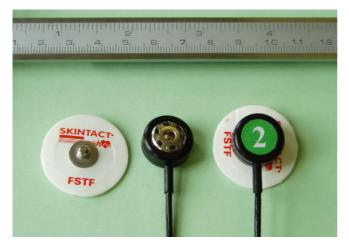
Fig. 2. Active electrode formed by a disposable Ag-AgCl electrode and active adapter with a snap connection and a special multi-wire cable
