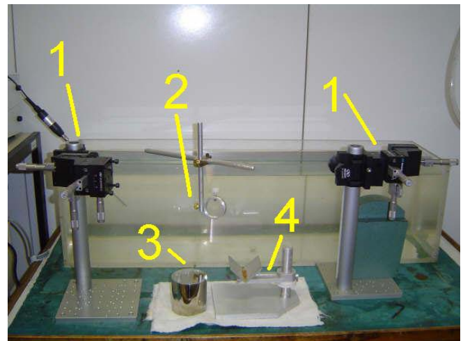
Fig. 1. Reciprocity calibration facilities: 1. Micro positioning systems; 2. Transducers holder; 3. Stainless steel reflector target; 4. Target bed. The acrylic water tank is in the figure background.
