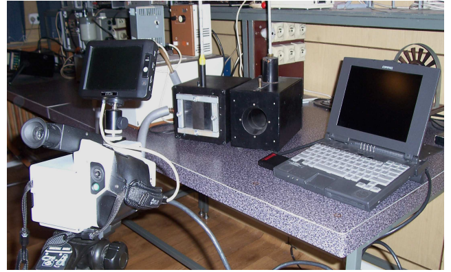
Fig. 1. The equipment for the measurement of the effective emissivity
