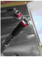
Fig. 7. Small magnetic socket on the sensor tip
