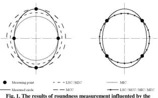
Fig. 1. The results of roundness measurement influented by the distribution of the measuring points and different fitting methods
