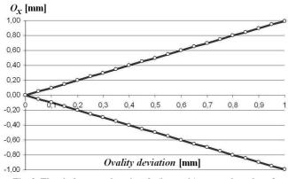
Fig. 3. The circle center location  $O_x$  (in x-axis) versus the value of ovality deviation
