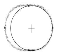
Fig. 2. Measurement of the circle with ovality deviation usin 4 points
