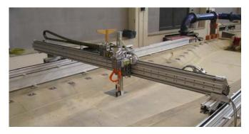
Fig. 6: Measurement device over model
