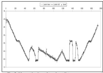
Fig. 5: Measured values of two laser-distance sensors compared with classically leveled values
