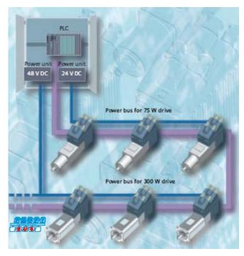
Fig. 8: Connection of POSMO A drive in control loop
