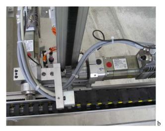
Fig. 7: Toothed belt drive for X-axis (a) and gear drives for Y and Zaxis (b).
