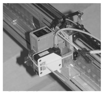
Fig. 3: Laser-based distance measurement instrument
