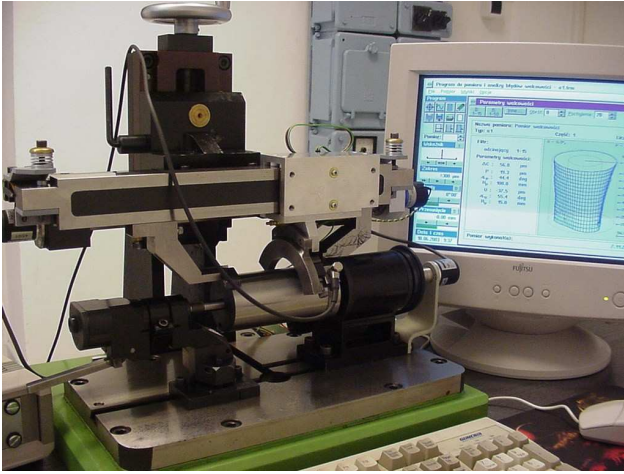
Rys. 2. A model test measuring device for V-block measurement of cylindricity profiles PSA 6
