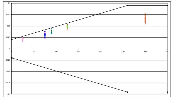
Fig. 6. MPE for adapted robot COMAU SMART 3S – after correction (using built ANN model)
