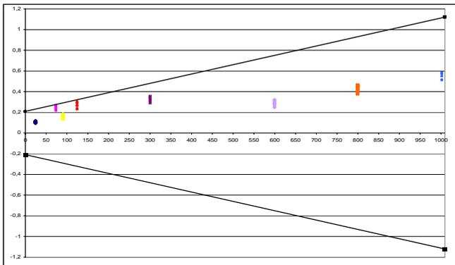
**Fig. 8. MPE for adapted robot COMAU SMART 3S determined using a KOBA-step artifact – after correction and extending corrected space**
