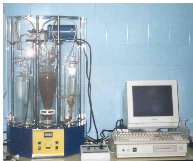
**Photo 1** Picture of lab-scale wastewater treatment plant
