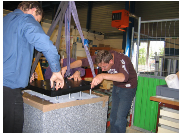
Fig. 5. . Installation of the exciter interface plate on the new 1200 kg block
