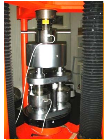
Fig. 7. Calibration of the INRIM – 3 MN Build-up system on the INRIM – 1 MN DWM
