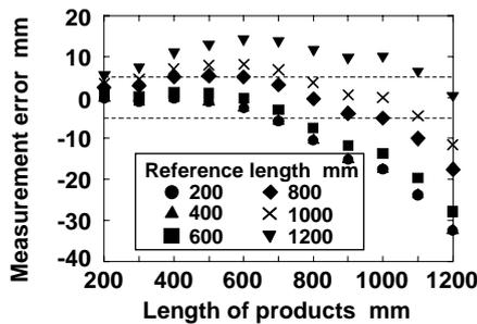
Fig. 7. Relation between estimated error and reference
