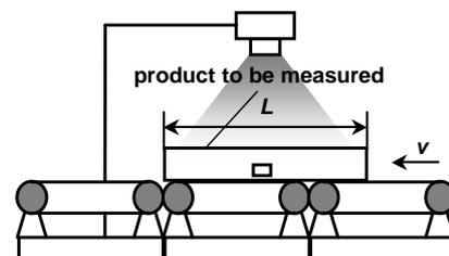
Fig. 1. Length measurement system
