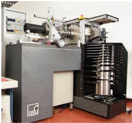
Fig. 3. 1 kN·m torque reference standard machine in the HBM calibration laboratory
