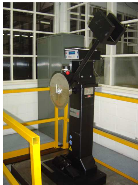
Fig. 1. Instron Impact testing machine DI-300
