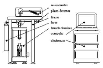
Fig. 1. Simplified scheme of the IMGC-02 absolute gravimeter
