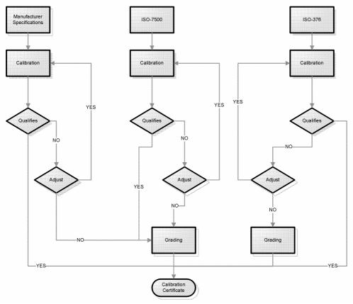
Figure 1: Flow chart of force calibration procedure in QCC Hazorea
