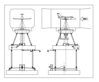
Fig. 2 - TA-2 external balance.  $R_1, \ldots, R_6$  represent load cells.
