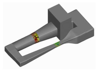
Fig. 1: The TA-2 wind tunnel.
