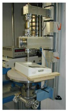
Figure 4 - View of the 50 N·m torque reference device with a Torque tester as calibration object
