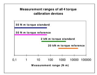
Figure 5 - Overlapping ranges of all laboratories torque calibration devices
