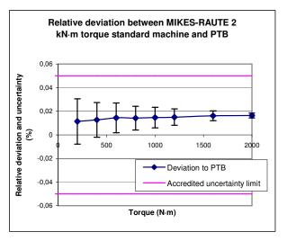
Figure 1 - Relative deviation and uncertainty of MIKES-RAUTE 2 kN·m torque standard device in comparison to PTB
