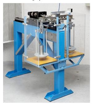
Figure 3 - View of the 50 N·m torque standard device before changing of the air bearing
