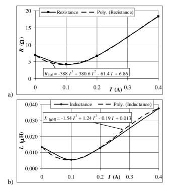
Fig. 2: The experimental results at 32 MHz for resistance - a), and inductance - b), of MI together with the corresponding trend lines used in simulation.
