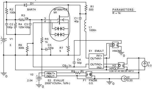
Fig. 4. Electrical diagram for PSPICE simulation
