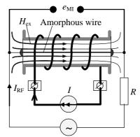
Fig. 1. The schematic arrangement of the current sensor
