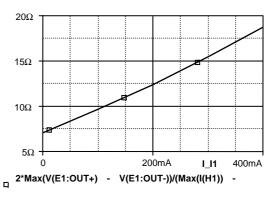
Fig. 7. Amorphous wire resistance variation vs. I1.
