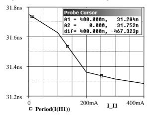
Fig. 8. Period of oscillation of the test current I<sub>H1</sub> vs. I<sub>1</sub>.
