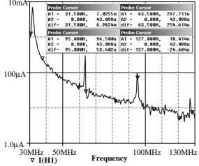
Fig. 9. Power spectral density of the test current  $I_{H1}$ ; parameter -  $I_1$ .
