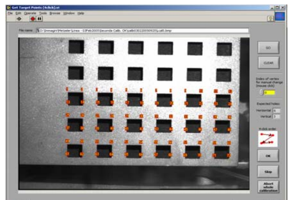
Fig. 3: Target corner detection during the calibration.
