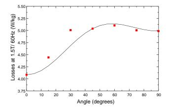
Figure 2 Experimental results for iron losses at 1.5 T / 60Hz (points) compared with equation (4) (full line).
