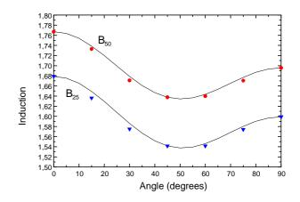
Figure 1 Experimental values for  $B_{25} e B_{50}$  (points) compared with values from equations (2) and (3) (full lines).
