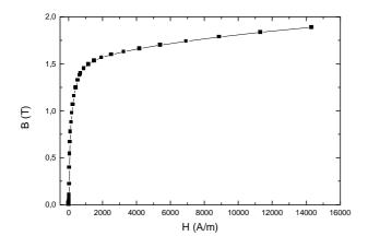
Figure 4. Initial magnetization curve measured in a ring.
