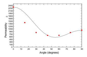
Figure 3 Experimental results for permeability  $\mu_{15}$  (points) compared with equation (5) (full line).
