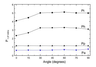
Figure 5. Losses - total, hysteresis, eddy and anomalous as function of the angle to RD. B=1.5T, f=60Hz. Epstein.
