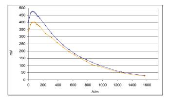
Fig. 9. hysteretic  $\lambda$ -H response in as-cast amorphous ribbon
