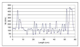
Fig. 4. Coercive field Hc versus ribbon length
