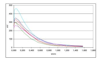
Fig. 8. The first derivative of the  $\lambda$ -H response at various points of a stress current annealed wire
