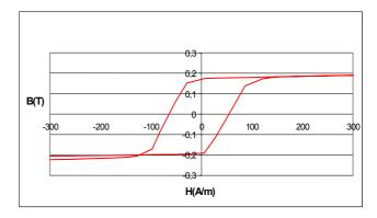
Fig. 3. Typical B-H loop for a stress-current annealed amorphous fiber
