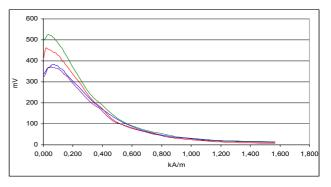
Fig. 7. The first derivative of the  $\lambda$ -H response at various points of a stress current annealed ribbon
