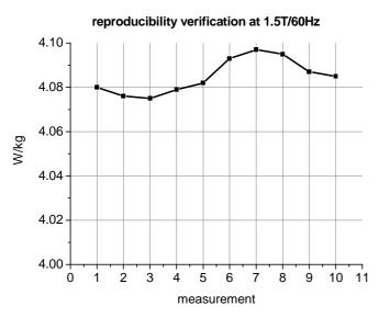
Figure 2. Losses at 1.5T/60Hz for reproducibility verification
