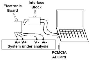
Fig. 4. Block diagram for the measurement setup.
