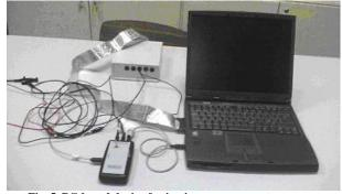
Fig. 5. PC-based device for in vivo measurements.
