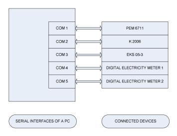
Fig. 3. Connection of the devices to the master PC.
