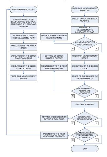
Fig. 6. Flowchart of the program Station - automated measurement.
