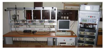
Fig. 2. Photograph of the calibration laboratory with electronic calibration station EKS 05-3.
