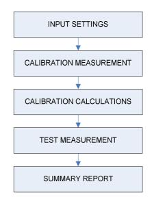
Fig. 4. Steps of the automated calibration process.
