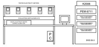
Fig. 1. Schematic drawing of the calibration laboratory with electronic calibration station EKS 05-3.
